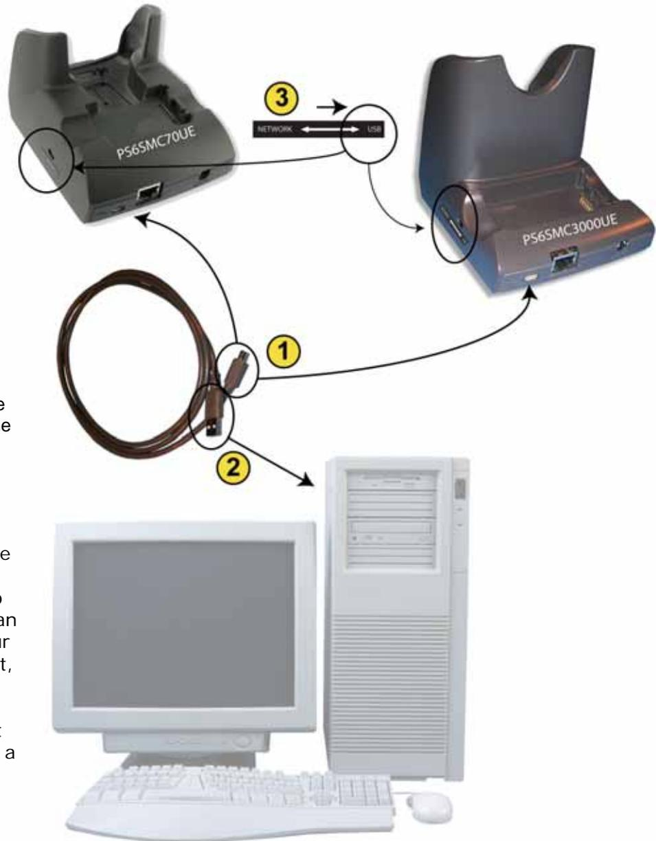
Once you have the cradle connected to the host device, insert the handheld terminal into the cradle. Now you can communicate with your host device to transmit, or synchronize, data. You can even browse the internet if the host device is connected to a network with internet access.
